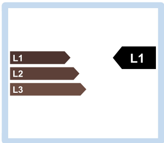
Casing leaky class at 400 Pa EN 1886 (M)
